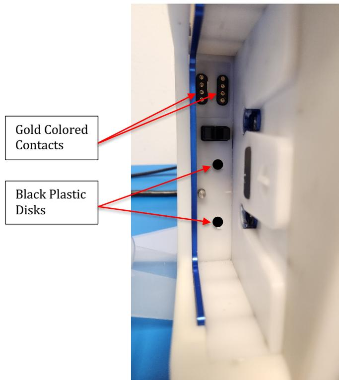
4. Wipe the Console again with a clean, soft cloth dampened with tap, distilled or sterile water to remove any detergent residue. **DO NOT** press down on the black circular disks in the Cassette Dock. **DO NOT** wipe the gold-colored contacts in the Cassette Dock.
