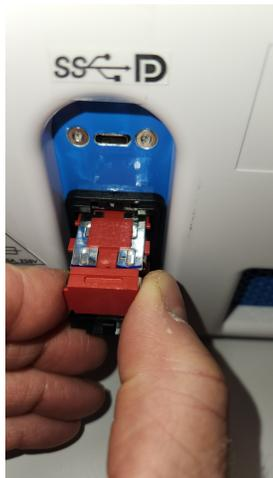
Insert the head of a small flat head screwdriver under the end of each blown fuse. (Note: there are 2 fuses). Gently lift up the end of the fuse and remove.
