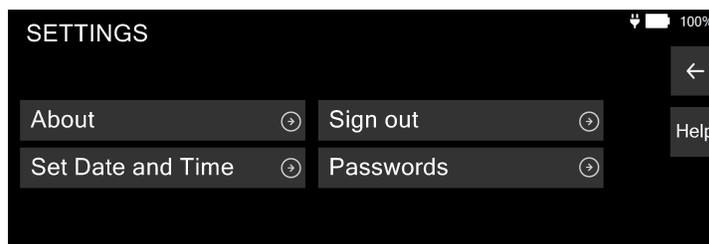
The “Settings” Screen provides the capability to see the software version, set date and time, sign out from the system, and change the user passwords. To view the system software version and revision, select “About” from the Settings Screen. The Settings Screen can be accessed from Home Screen by pressing
