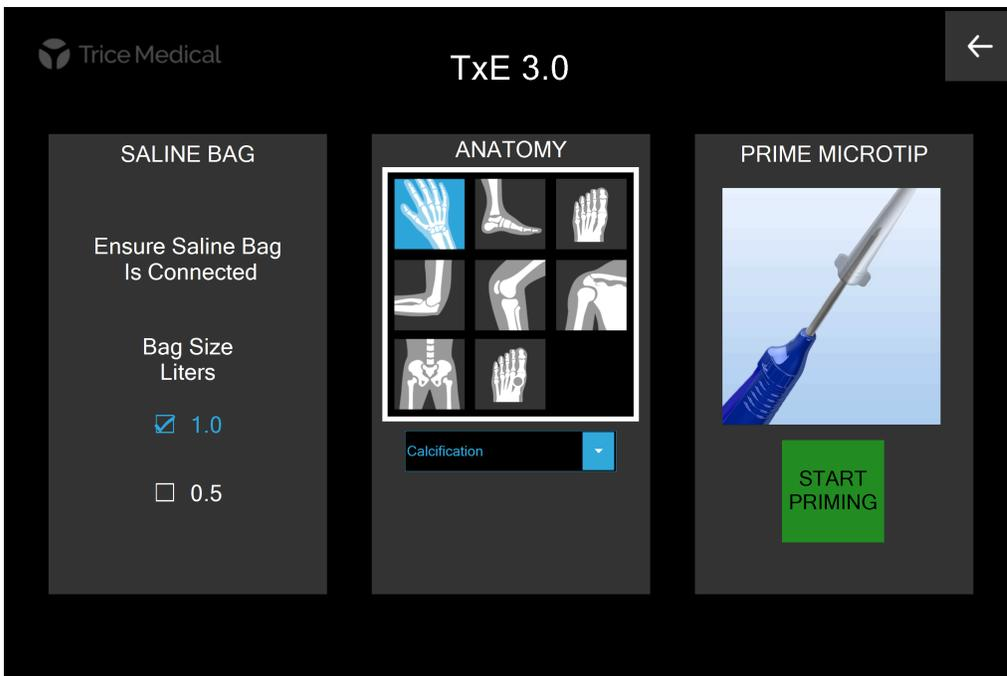
On the Priming Screen, select the size of the Saline Bag, “Anatomy,” and “Sub-type” from the dropdown menu and “Start Priming” to prime the system.
