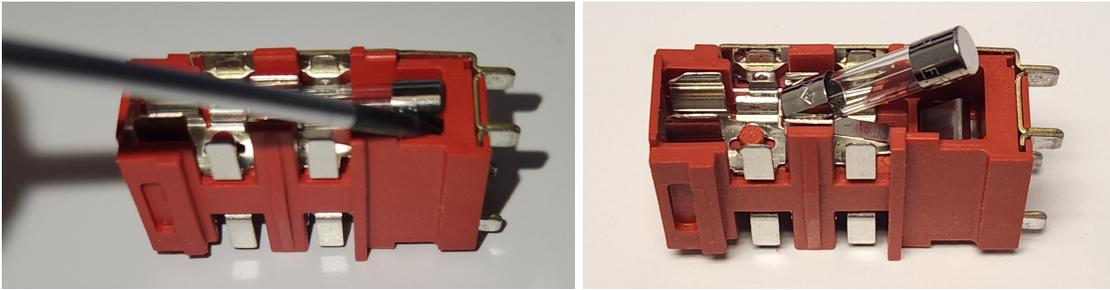
Replace the blown fuses with Slo-blo (Time Delay) 5mm x 20mm 2.5A, 250V fuses as specified in the accessories table in Section 2.1 Contents and Accessories.
