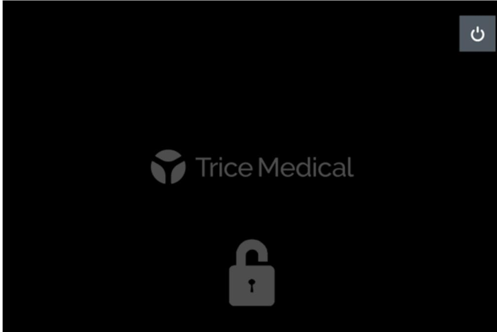
To lock the Console screen when not in use, press the “Lock Screen” button
