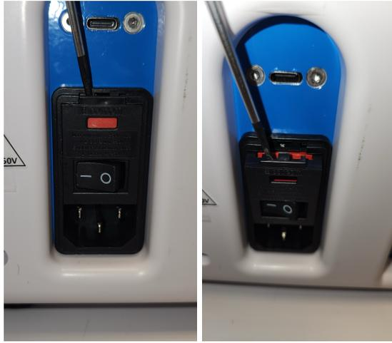
Insert the head of a small flat head screwdriver between the top of the red colored fuse holder and the housing of the appliance inlet. Pry out the fuse holder to slide it out.
