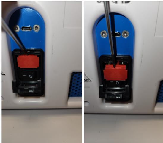
Remove the fuse holder noting its orientation.
